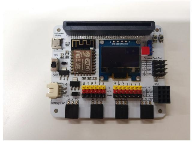
Smarthon IoT:bit is an WiFi extension board for micro:bit. With input/output ports, we can obtain information from different sensors for IoT and control the actuator (such as LED lights and servo)
